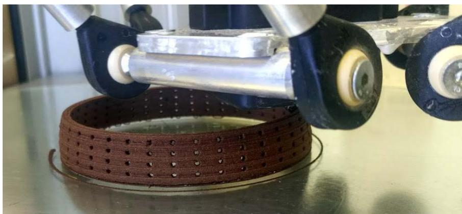
*Fig. 5 Model of printing a cork studied coil.*
