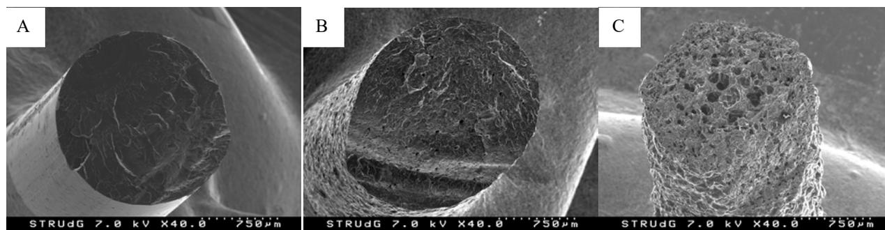
Fig. 3 SEM micrographs of PLA coil (A), cork commercial coil (B) and cork studied coil (C).
