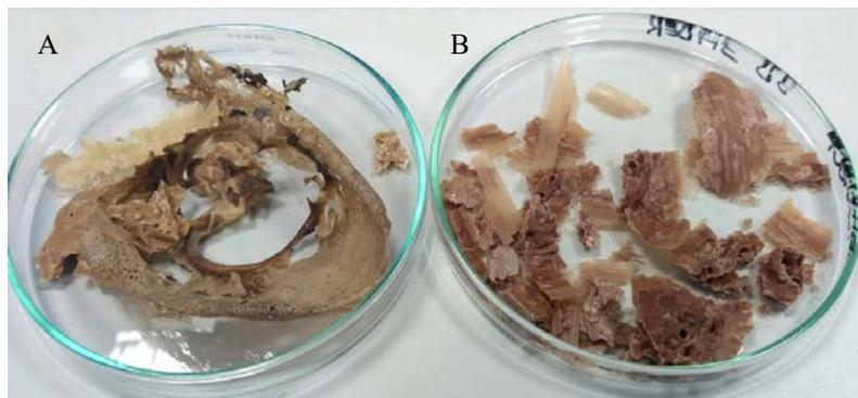
Fig. 1 Dichloromethane extractives content in commercial (A) and studied coil (B).
