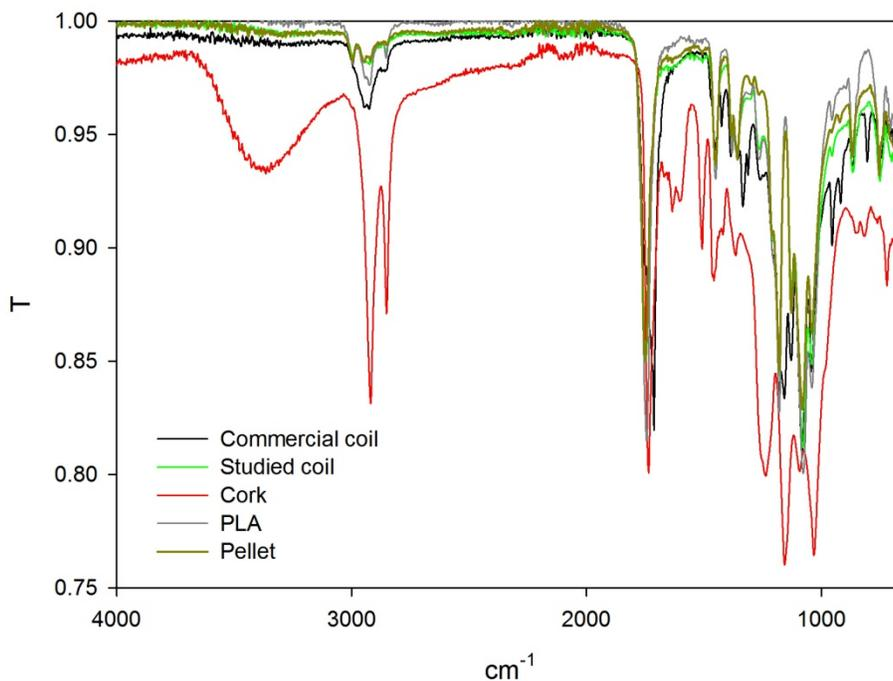
*Fig. 2 FTIR spectra of cork, PLA, studied cork coil and commercial cork coil.*
