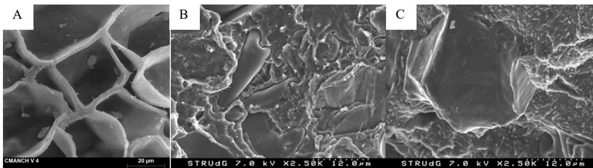
Fig. 5 SEM micrographs of cork (A), cork studied (B) and cork commercial (C).
